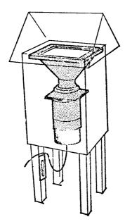
Note 1—The clearance area between the main housing and the roof at its closest point should be  $580.5 \pm 129.0 \text{ cm}^2(90 \pm 20 \text{ in.}^2)$ . The main housing should be rectangular, with dimensions of about 290 by 360 mm (11½ by 14 in.).
